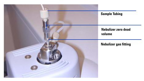
Figure 18 Nebulizer with gas tubing connected
